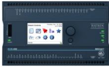
The ECB-450 and ECB-453 have a large color backlit-display that allows an operator to have immediate access to internal controller data.
