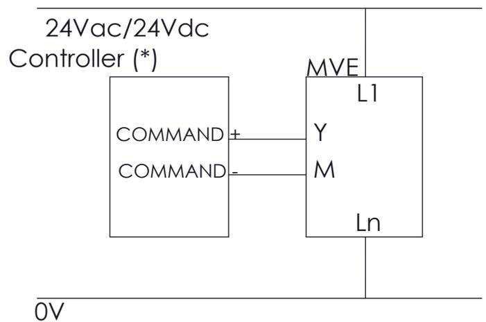
N.B.: M and Ln signals are internally connected.
