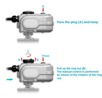
The lowered ring allows the reduction of the overall dimensions of the actuator. Once extracted facilitates the rotation thanks to a larger area of grip.
