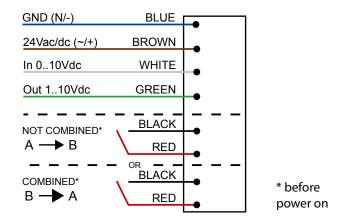
If before powering the system, the BLACK and RED wires are connected together, you will get B as the starting position of the actuator, while if left disconnected (factory condition) you will get A as the starting position.
